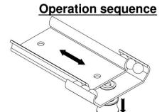
To lock, the spring-loaded handle is released. To loosen, the spring-loaded handle is pulled out.
