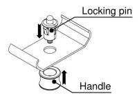
To install, the locking pin is simply pushed into the cutout without the use of tools or hardware. The handle slides over the housing and secures permanently into the groove of the pin.
